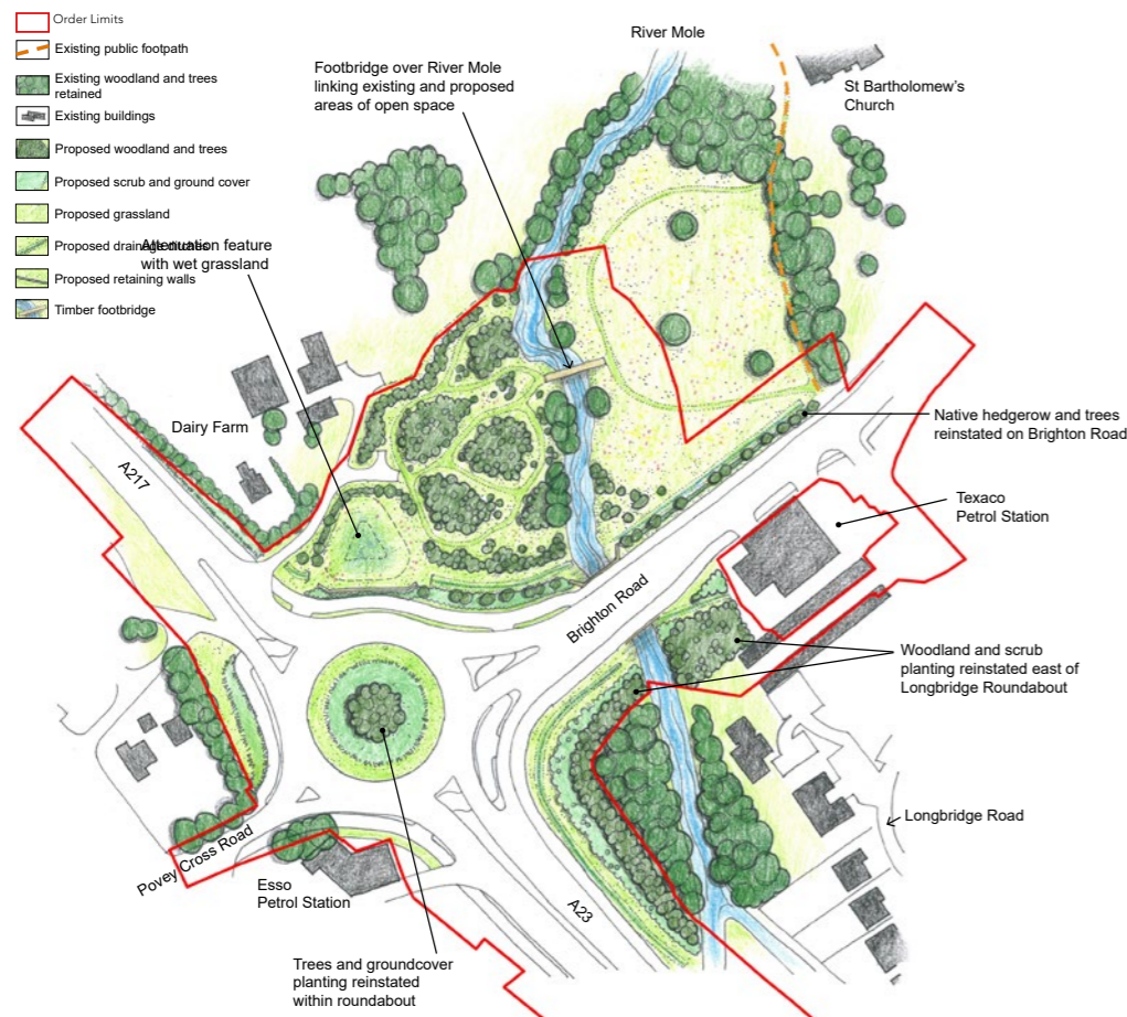
Figure 66. Indicative plan of Longbridge Roundabout showing how the design has been integrated into the surrounding landscape, ES Appendix 8.8.1
